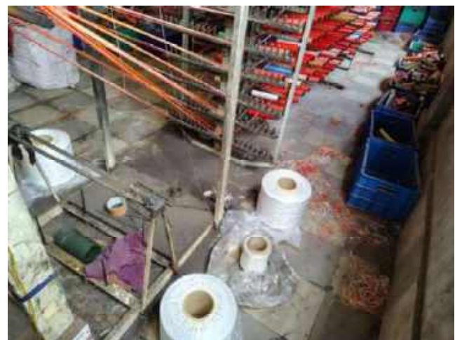
PLASTIC TAPE / RASSI PLANT INTAKE SECTION WITH BOBBIN AND BINDING PLASTICE WIRE REEL WHITE COLOUR.
