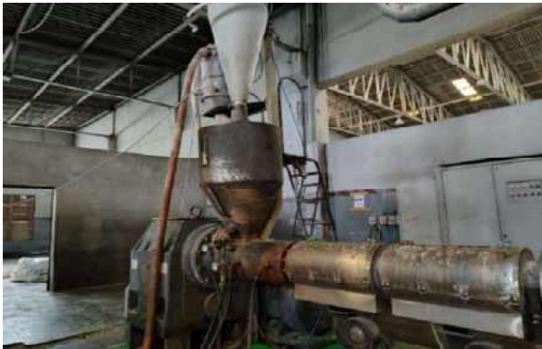
Hopper/extruder barrel tape plant
