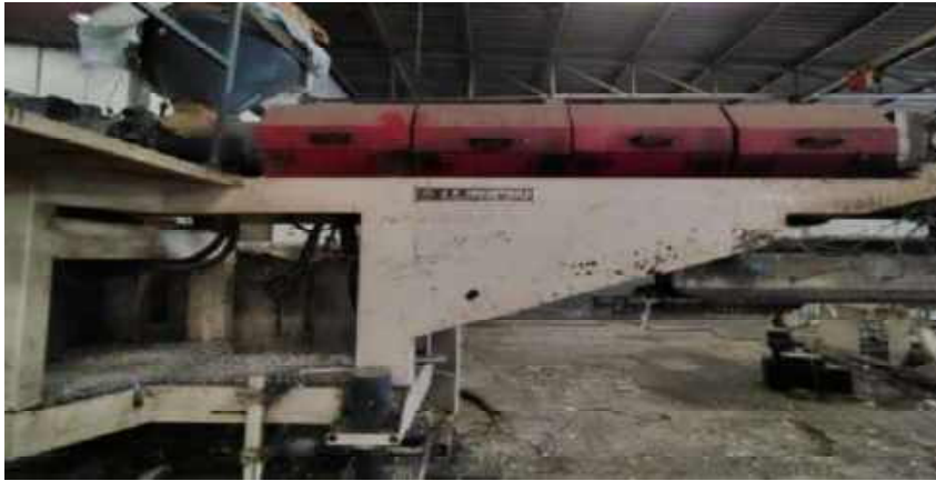
Heating barrel of sealing film unit
